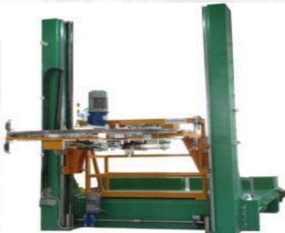
TRANSFORMER CORE TAPING MACHINE
